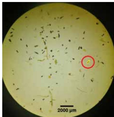
Figure 1: Supervised analysis of charcoal using edge-detection from CharTool v1 macro in ImageJ. Users select a charcoal fragment, then the algorithm draws an outline around the fragment and calculates measurements (Image credit: Enele Twala).
